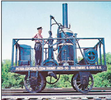
Tom Thumb, first American steam engine in regular service
